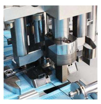
Ear with welding: the use of high-pressure device to prevent deflection; titanium alloy welded joints, durability, and excellent welding results.
